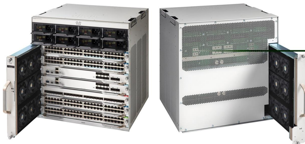
Figure 2. Dual serviceable fan tray
